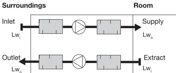
The flow noise and pressure loss is dependent on the velocity ( $v$ ) on the face area( $A$ ) of the attenuator.
