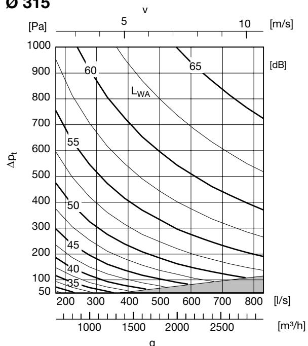
The grey area in the graph shows the minimum pressure drop needed for the product to start working. Even if the damper blade is fully open you get this pressure drop measured over the product.
