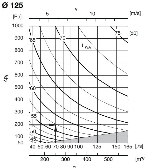
The grey area in the graph shows the minimum pressure drop needed for the product to start working. Even if the damper blade is fully open you get this pressure drop measured over the product.
