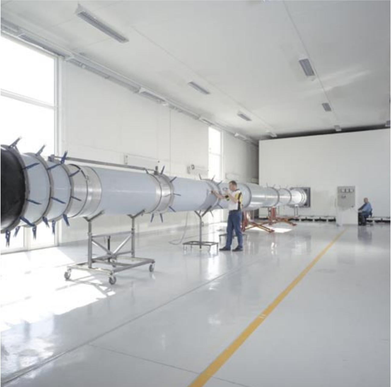
*21 metre measuring duct. Here it is possible to install both circular and rectangular silencers.*
