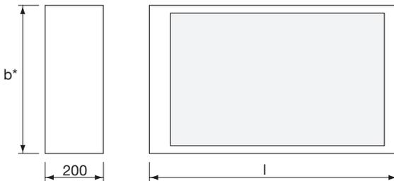
b\* = Manufactured height of splitter is b-5 mm, to fit into duct.
