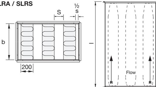
See how to calculate (S) from a given (a) in the separate AeroDim-SLRA-SLRS installation instruction page 4.
