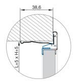
When using the MFA for installation, the cutt-out dimension must be 5 mm larger than the nominal L x H dimension.
