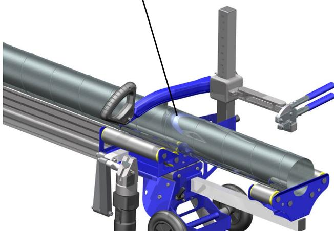
1. While moving the arm downwards turn the handle so that the knife protection is retracted
