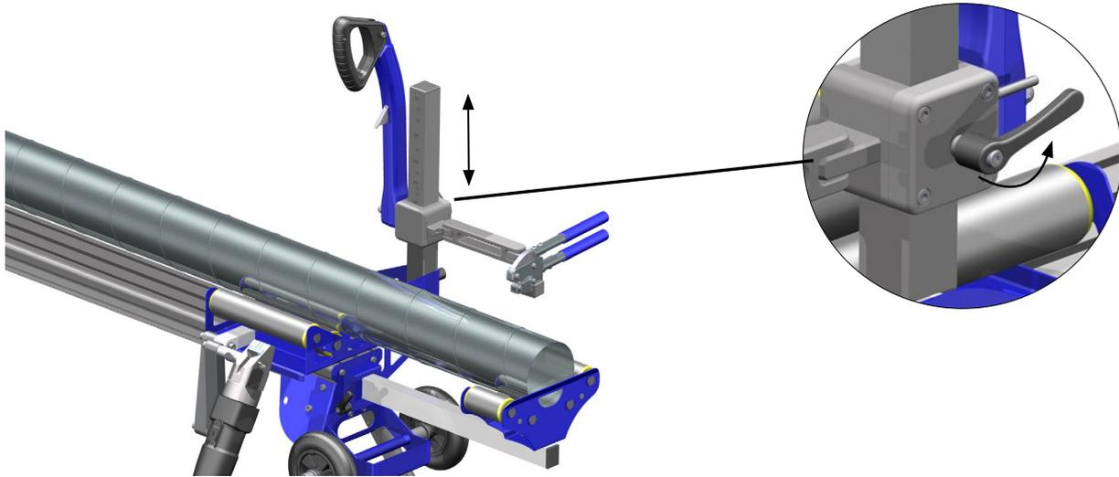
1. Loosen the locking handle on the setting block.
