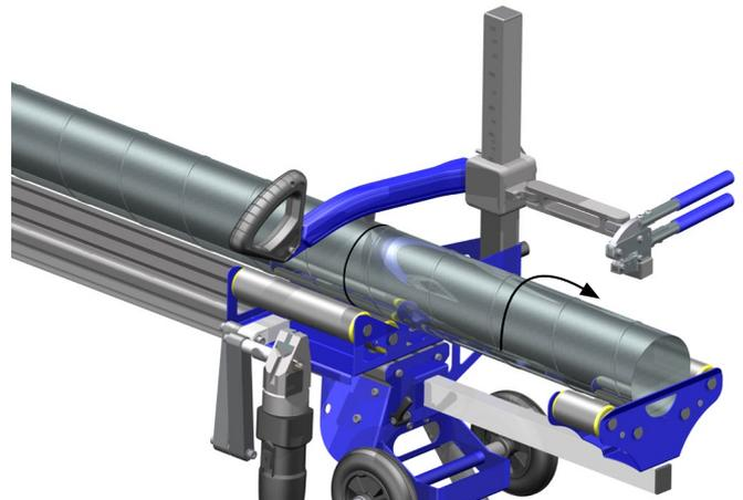
1. Scratch a thin line with the point of the knife around the duct. The easiest way to do this is turning the duct away from you.
