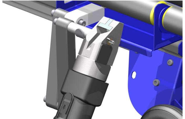
1. Turn the split pin so that it is possible to mount the shears onto the arm.
