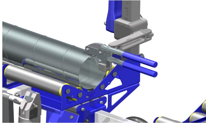
1. Insert the opening of the pliers over the duct end as far as it can reach.
