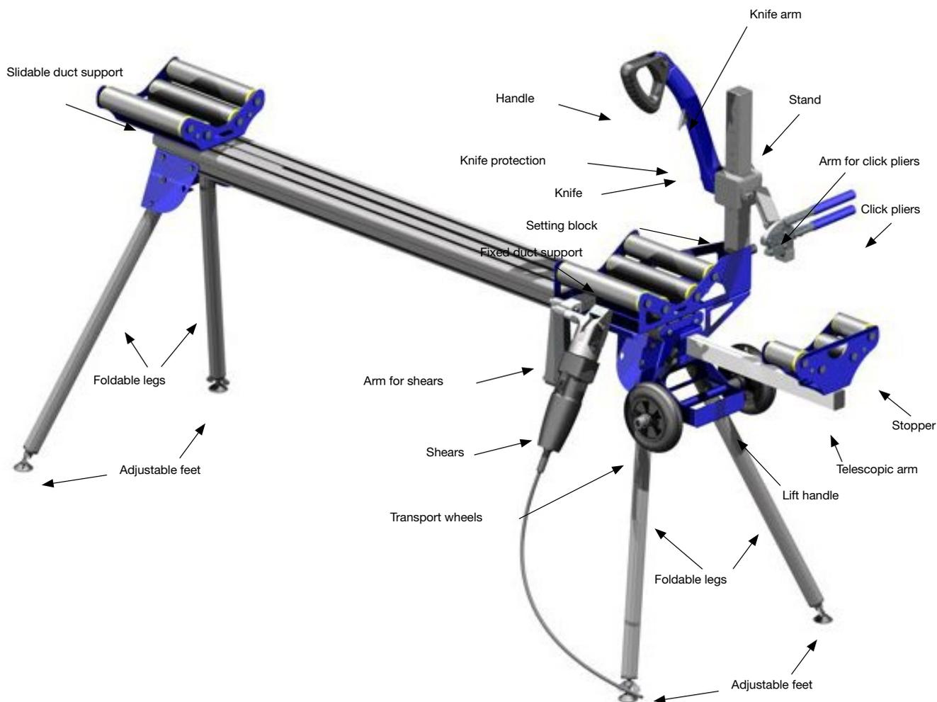
With this workbench you can cut ducts of 80-315 mm diameters and lengths of 200 mm and upwards.
