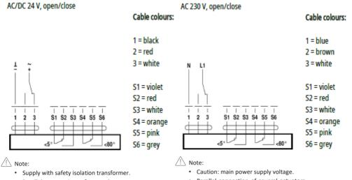
Parallel connection of several actuators possible. Power consumption and switching thresholds must be observed.
