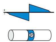
Since ps will be negative in relation to atmospheric pressure (on the suction side of the fan), this means that pt will also be negative if the total of  $p_{\rm S}$  and  $p_{\rm d}$  is negative.
