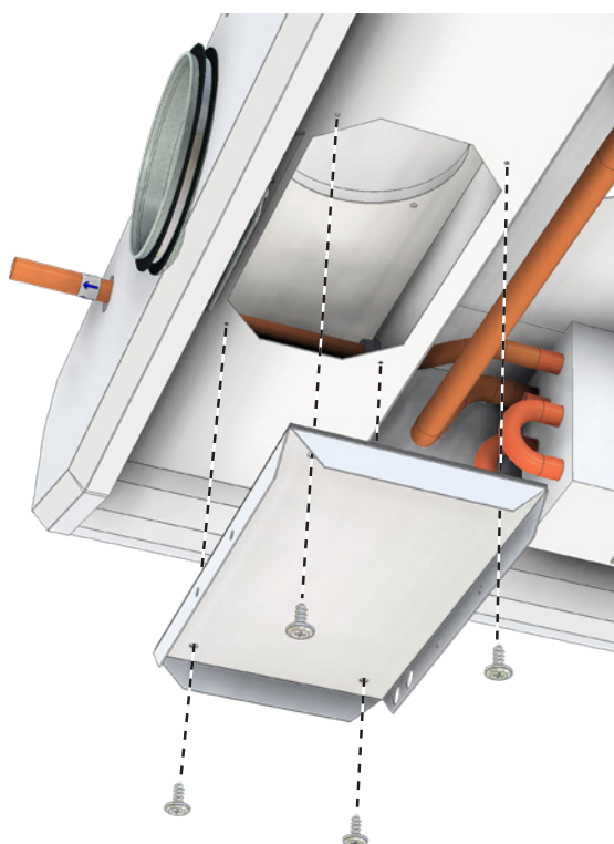
Picture 20. Opening inspection hatch.
