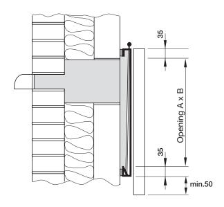
The accompanying installation rail should be fastened to the wall. The fresh air valve is suspended from the rail and fastened to it by means of screws through the lower edge of the front plate.
