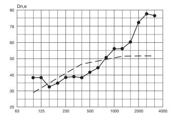
The sound insulation measurements were undertaken by DELTA & Vibration, in accordance with the testing instructionsin DS/ISO 140-3:1978.
