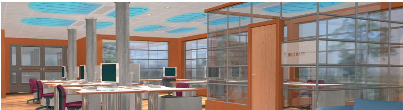
Picture 6. A separate office is to be fitted into the room. If the climate is to be optimal, the air quantity and air volume need to be adjusted for the Premax beam that will be built into the new room.
