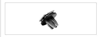
The small Vane Fastener is used for sheet steel thickness 0,75–0,9 mm.  $\,$
