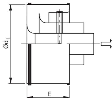
Concentrated supply air – for installation in a circular duct or fitting. The insert is turned 180 degrees.
