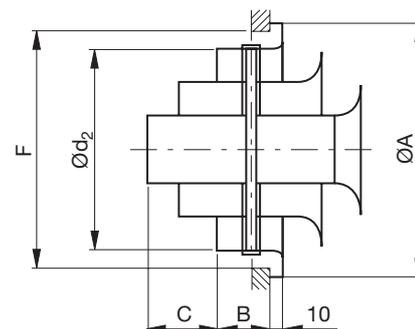
Diffused supply air – for installation in a wall or duct side. Remove the external pipe.
