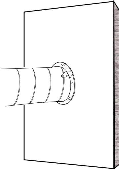
1. Press the flange up against the wall / deck and attach it to the duct using brackets type VINKE60.
