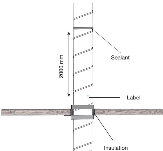
On all joints within 2000 mm from penetration, vertical ducts must be sealed with sealant BSKTUBE.
