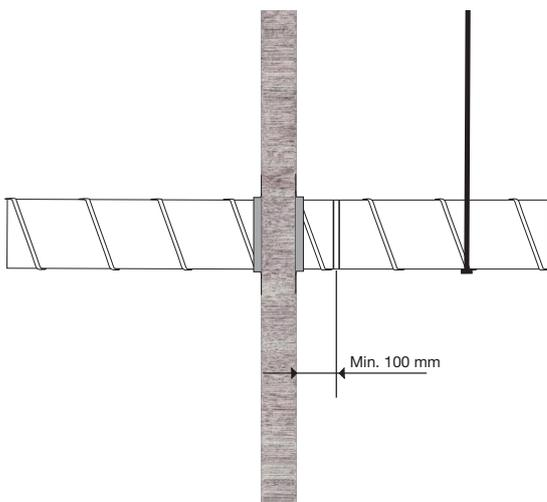
Distance from wall, deck or ceiling penetration to first duct joint must not be less than 100 mm.
