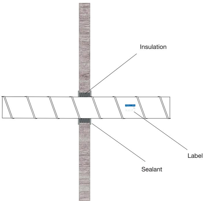
1. Place the duct in the hole of the wall / concrete deck. The gap between the wall / concrete deck and the duct must not exceed 25 mm.
