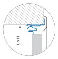
The grille is installed on the MFS by clips .
