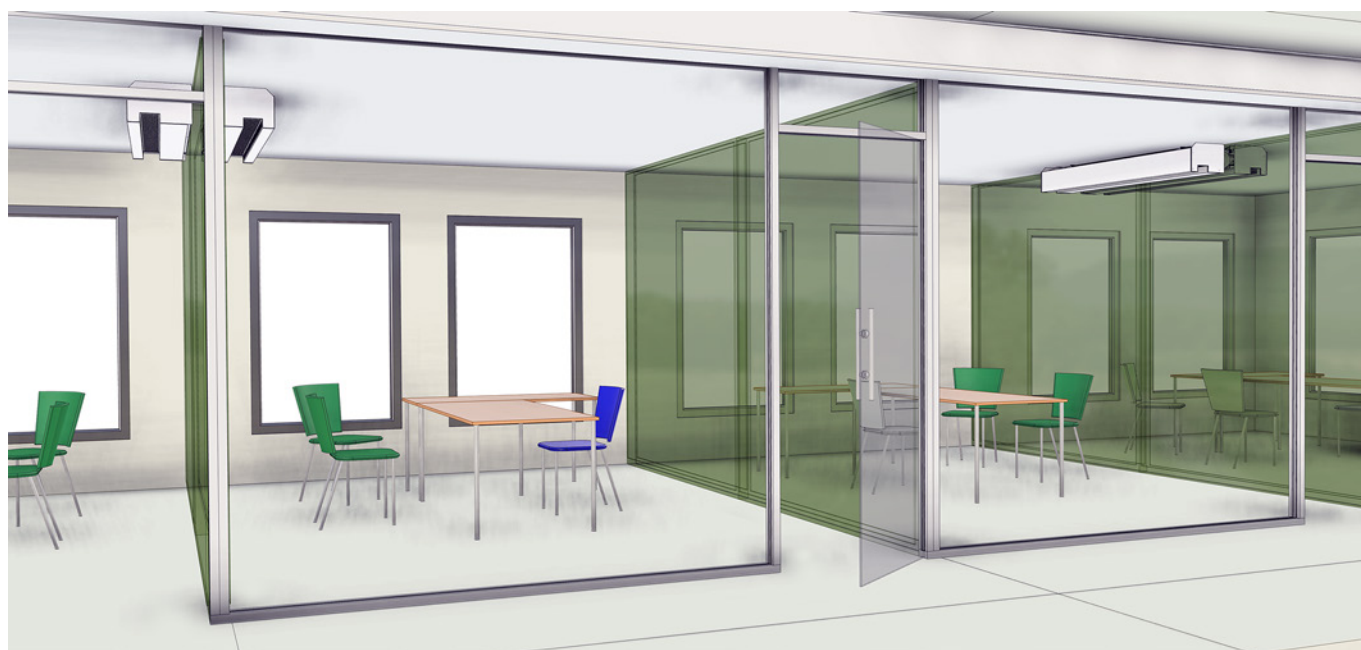
Picture 52. Plafond XD mounted back to back around removable partition wall, sealed to the ceiling.
