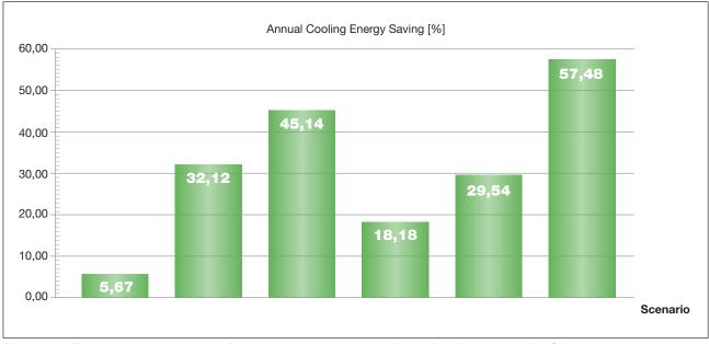
Diagram 3. Energy saving percentage for the energy demand, cooling only, when comparing Solus and a conventional chilled beam system.
