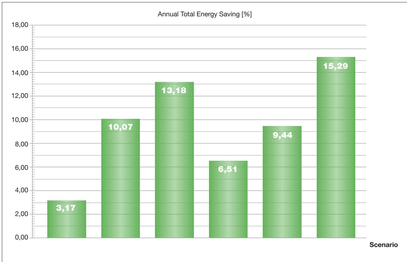
Diagram 2. Energy saving percentage for the total energy demand, heating and cooling, when comparing Solus and a conventional chilled beam system.
