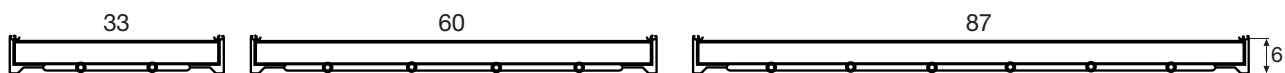
Figure 5. Atrium and Loggia are manufactured as standard in three widths, 33, 60* and 87 cm, and one height, 6 cm. Actual width dimension is -8 mm.
