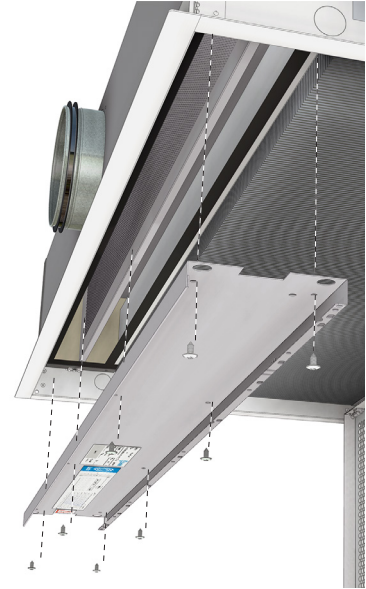
Picture 5. Cleaning hatch off.
