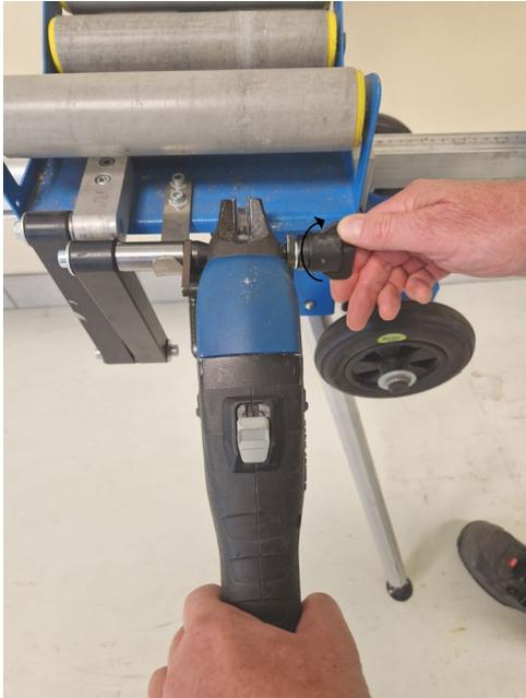
5. Secure the shear by tightening the knob.
