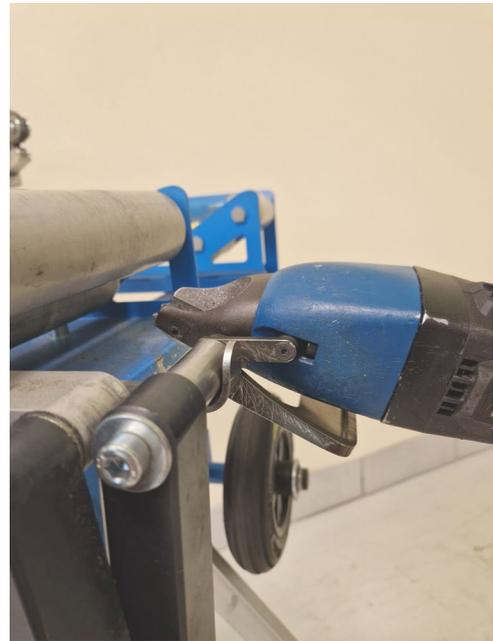
4. Mount shear TRC200 onto the adapter.
