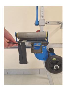
3. Secure CSAD with the locking bolt.
