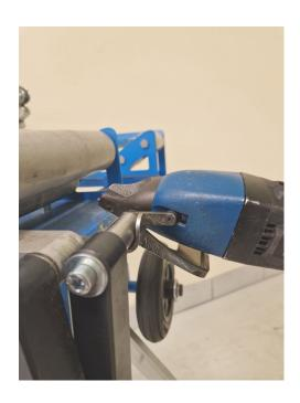
4. Mount shear TRC200 onto the adapter.
