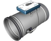
Two flow sensors are mounted on the sensor body and connected to a display unit via cables. The display unit is mounted on top of a shelf on the sensor body.
