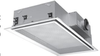
Plexus is provided with fixed lamellas which controls the primary air into non-parallel jets in a 360 degree air pattern. The 360 degree air pattern results in shorter air throws (30%) and a draft free indoor climate. Plexus can be used for both cooling, heating and ventilation. Plexus can be equipped with the functions Regula Secura condensation guard, down fold battery for better accessibility, and pre-mounted valves and actuators. The possibilities are many and the flexibility large.
