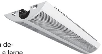
Architect can be equipped with cooling, heating, ventilation, Regula Secura condensation guard, built-in valves, actuators and built-in lighting.
