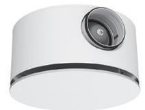
The LCFV includes a a unique linear cone damper with integrated volume flow regulator. In Pascal systems the LCFV is controlled by a Regula Combi room controller. LCFV is as standard delivered with a specially designed Regula connect card, for easy and simple wiring.
