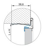
When using the MFAN mounting frame, the cut-out dimensions are the nominal dimensions of the grille (L x H).
