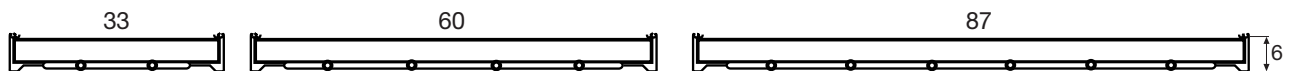
Figure 5. Atrium and Loggia are manufactured as standard in three widths, 33, 60* and 87 cm, and one height, 6 cm. Actual width dimension is -8 mm.
