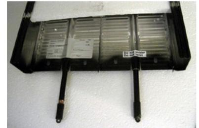
**Loggia** Fig.2: Label location interior (Under insulation, above water connection).
