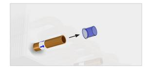
After removing the protection cover, make sure that the pipe is intact and undamaged, especially at the pipe end, as even small dents and scratches potentially pose a risk of leakage in the system.
