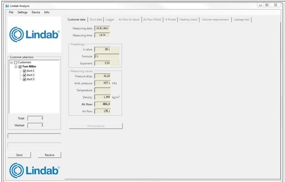
Fig. 18: Measurement mode "Air flow (k value)"
