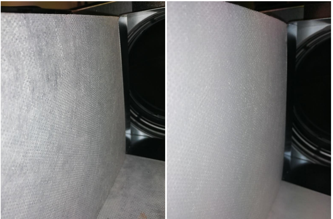
Figure 10. 90° elbow: 10 brush cycles: KVDPX-2 no2 and KVDPX-4 no2.
