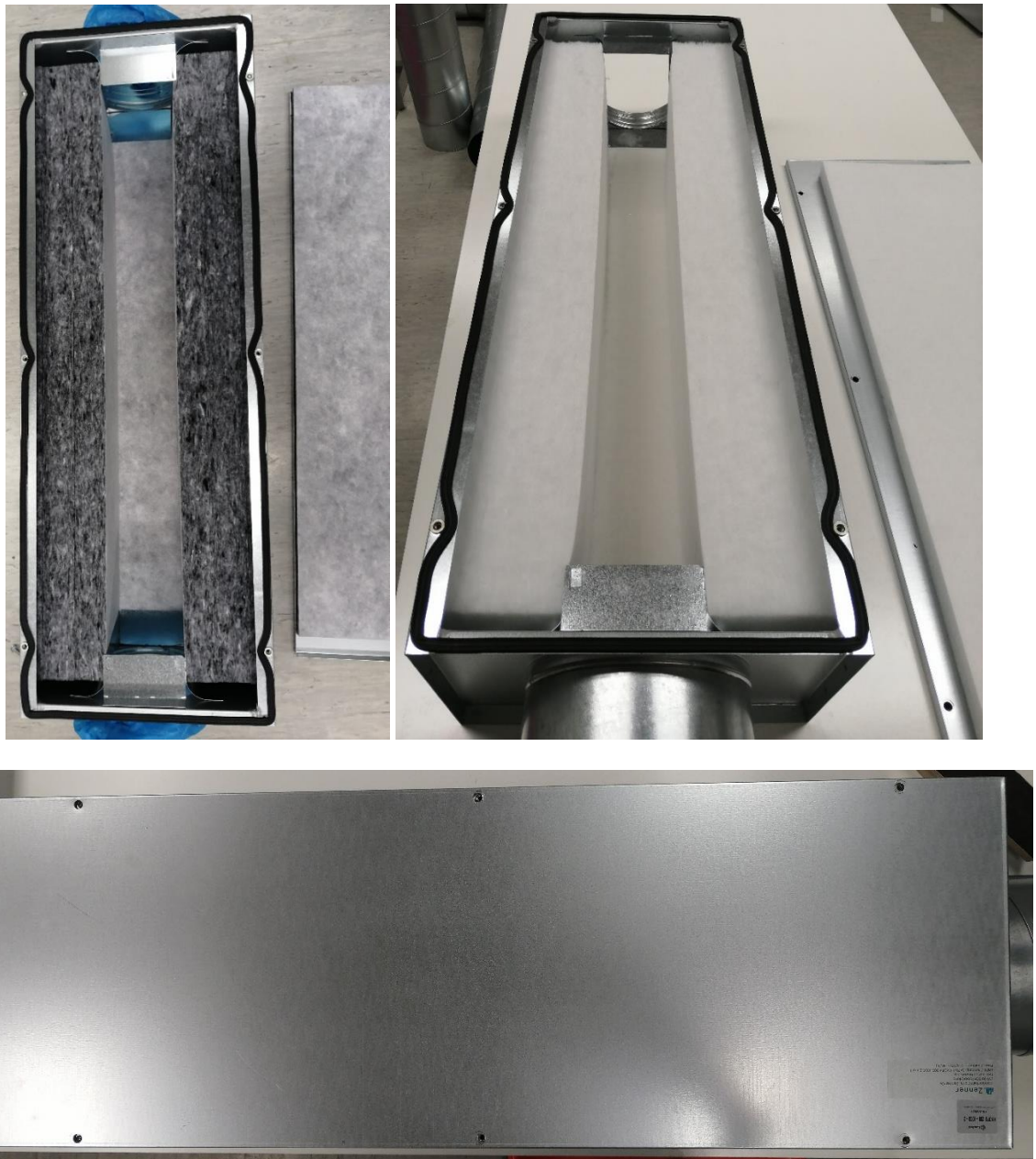
Figure 1. Measured silencers. In the top left picture model KVDPX-200-1000-2 (grey sound absorption material). In the top right picture model KVDPX-200-1000-4 (white sound absorption material). In the bottom picture a silencer with the detachable cover attached.
