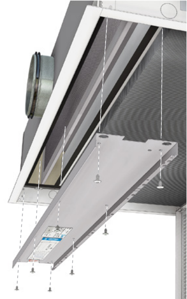
Picture 5. Cleaning hatch off.
