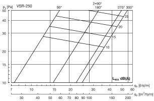
The sound levels from the nozzles apply for duct length 1 m.
