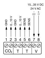
N.B. System neutral and signal neutral should be separately wired, because of current peaks in the supply wires. Screw terminal: Max. 1.5 mm<sup>2</sup>
