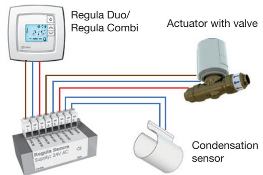
Schematic showing how to connect Regula Secura.
