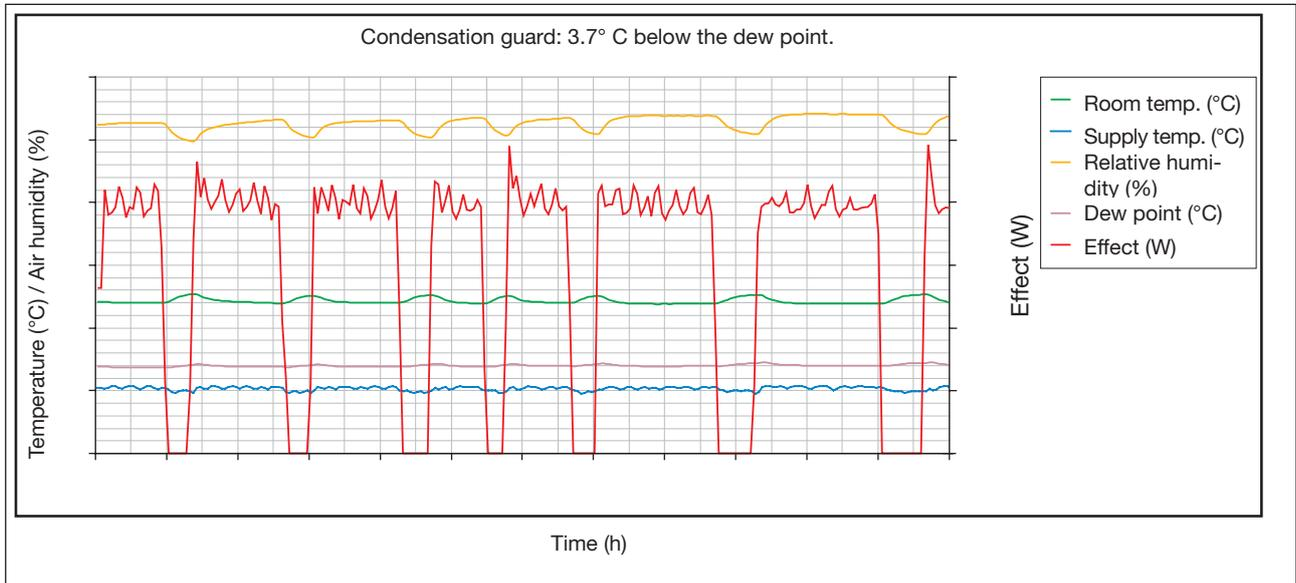
The diagram shows a control sequence where the water temperature is 3.7°C below the dew point. Throughout the whole process, the control centre asks for cooling. It can be seen how Regula Secura controls using the ON/OFF feature.
