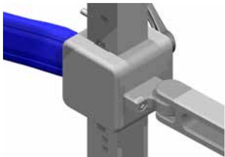
**EN** Mount the arm so that the pins fits into the holes in the setting block.
