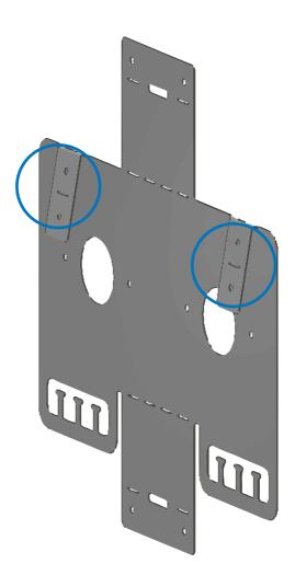
2. Bend the two larger parts 90° in the same direction as the two smaller parts.
