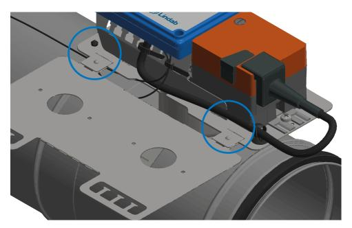
6. Bend the FTES so that it is positioned in a suitable angle to the FTCU.
