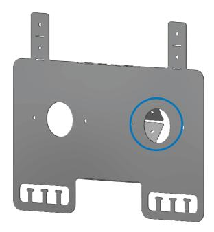
2. Bend the two smaller parts in the middle, in the opposite direction from the wide parts.
