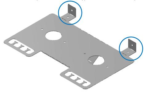
3. Insert the two small parts of the FTES into the slots in the FTCU's shelf from underneath.
