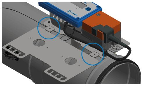
5. Attach rivets in the holes to fix the FTES in place.
