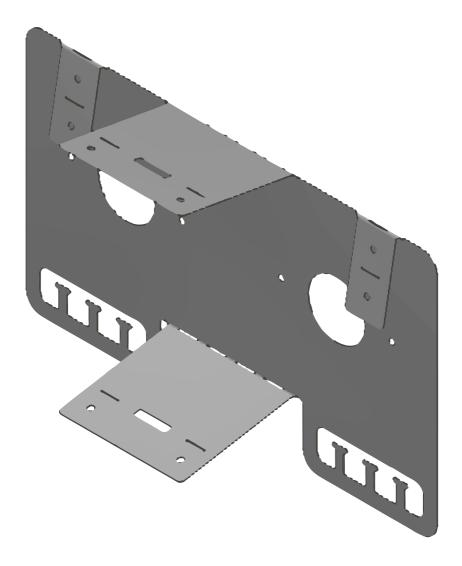
Bend the ends of the wide parts roughly 45° in the opposite direction. The angle depends on which dimension the FTMU is, for larger dimension an angle closer to 90° is suitable.
