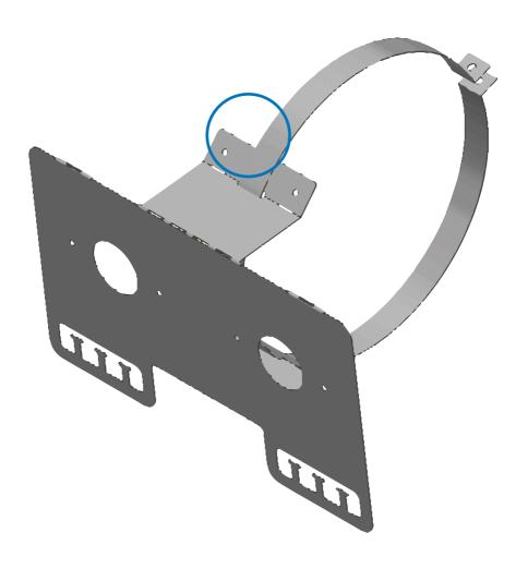
6. Run the strap through the slots in the display unit, then attach and tighten the screw. Both FTES and display unit should now be mounted roughly like the pictures below.
