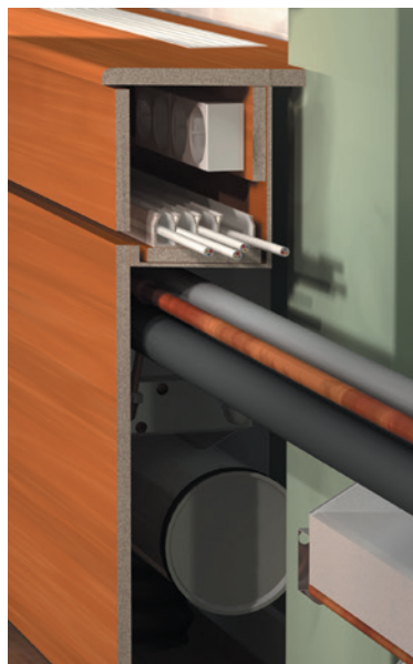
Picture 6. Casing with fixed worktop and detachable hatch on front side.
