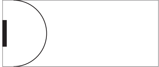
Fig. 21, Too great air flow on one diffuser results in a too big near zone.
