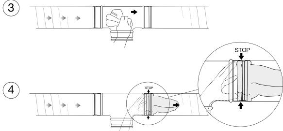
Thanks to this stop, it's not possible to press the filter too long inside the duct.
