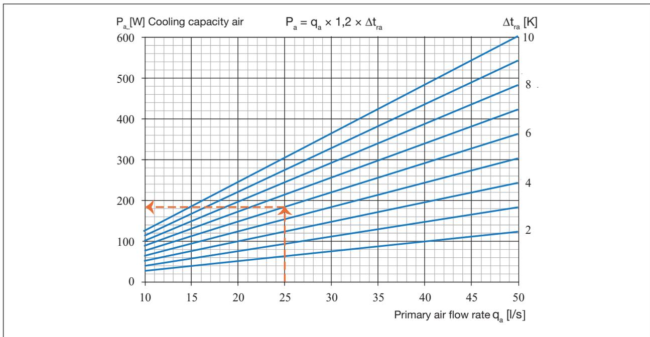
Diagram 1. Cooling capacity air  $P_a$  as function of the primary air flow rate  $q_a$ . If the air supply flow is 25 [l/s] and the temperature difference of the room air and the supply air is  $\Delta t_{ra} = 6$  K, then the Cooling capacity air of the air is 180 [W].
