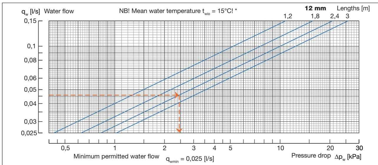
Diagram 4. Pressure drop in water circuit, cooling.
