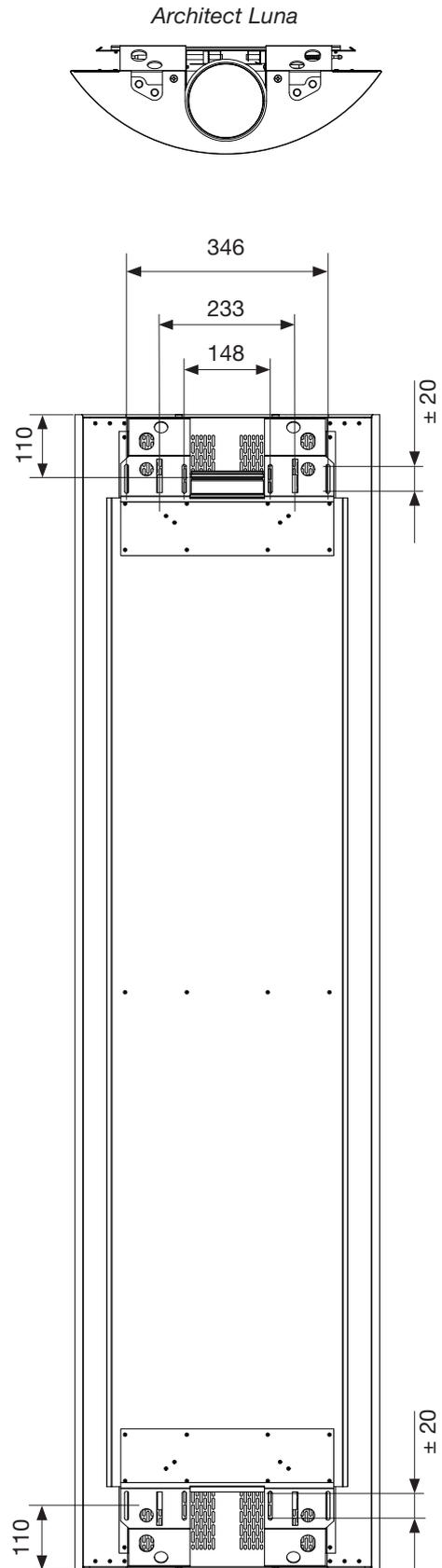
Figure 2. Architect Luna, Prisma and Circum, suspension / dimensions.
