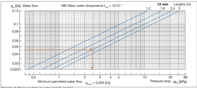
Diagram 4. Pressure drop in water circuit, cooling.
