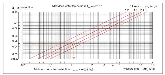
Diagram 5. Pressure drop in water circuit, heating.
