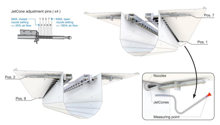
Picture 4. Architect Lindab's JetCone air volume adjustment system.
