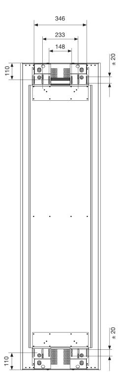
Figure 2. Architect Luna, Prisma and Circum, suspension / dimensions.
