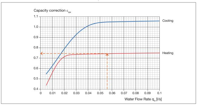
Diagram 3. Capacity correction  $\epsilon_{\mbox{\tiny aw}}$  for water flow for both cooling and heating.
