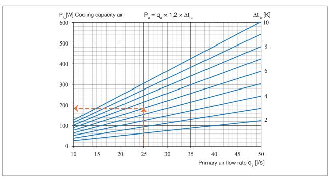
Diagram 1. Cooling capacity air P<sub>a</sub> as function of the primary air flow rate q<sub>a</sub>. If the air supply flow is 25 [l/s] and the temperature difference of the room air and the supply air is  $\Delta t_{ra} = 6$  K, then the Cooling capacity air of the air is 180 [W].
