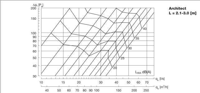
Diagram 6a+6b. Sound effect level  $L_{\scriptscriptstyle WA}$  at JetCone setting for Architect.
