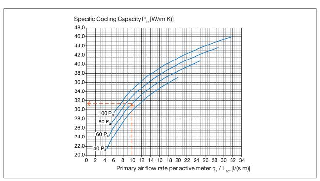
Diagram 2. Specific cooling capacity  $P_{tt}$  as a function of primary air flow rate per active metre at nozzle pressures of 40, 60, 80 and 100  $[P_{g}]$ .
