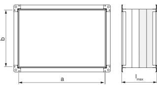
Minimum dimensions: 150x150 mm Maximum dimensions: 1900x1700 mm
