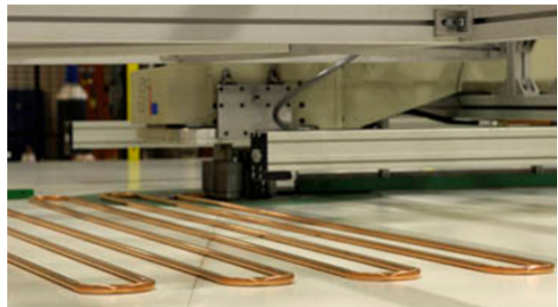
Picture 2: Atrium Plana high precision laser welding.
