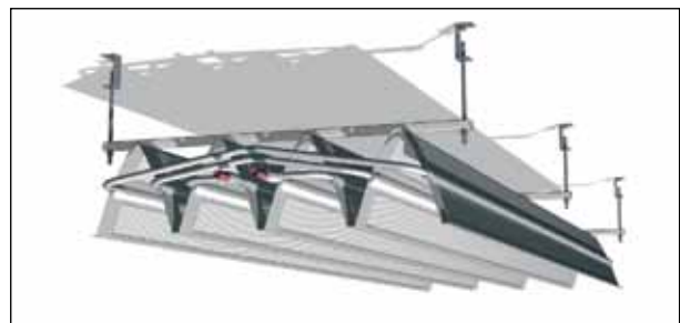
Picture 9. Installation of Carat with a threaded rod.
