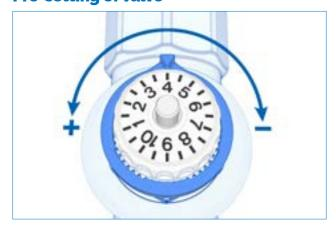
The KV value varies between the different valve sizes. See the pre-setting position for the desired value in the data sheet.
