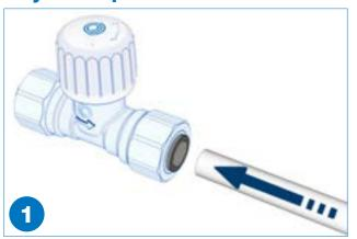
Prepare the pipe end with a deburring tool. 1 mm of the end should be angled at 30°. Push the pipe into the pipe stop.
