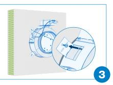
Fold the brackets against the wall and fasten them with screws and expanders.
