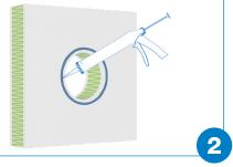
Seal with fire rated mastic between the wall and damper ring.
