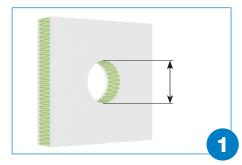
Cut a hole in the wall. Ventilation duct diameter +10 mm or +40 mm.
