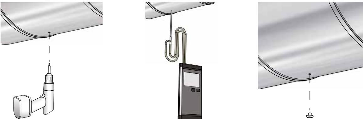
1. Drill a hole in the duct, about 3 times the diameter  $\varnothing$  of the duct, from the valve.
