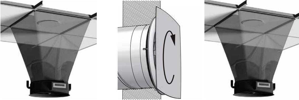
1. Place the flow hood over the valve and notice the air flow on the display.
