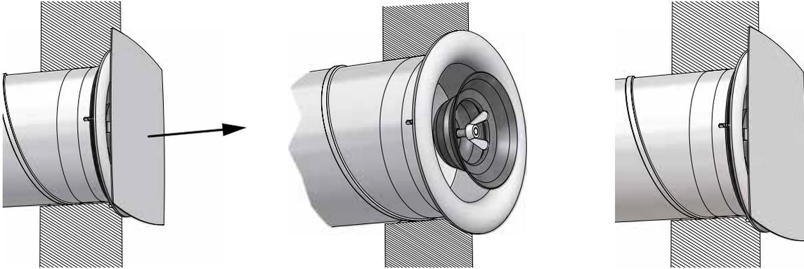
1. Remove the front plate and tighten the wing nut.
