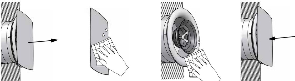
To clean the valve remove the front plate and clean it with a mild detergent or a wet cloth.
