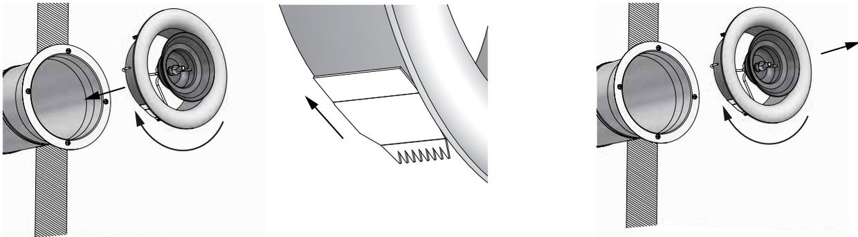
The valve is equipped with flexible spring wings intended to fit in sheet metal fittings.
