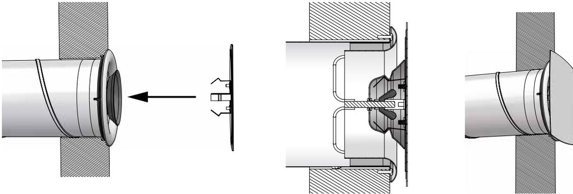
1. If the valve needs to be balanced do so otherwise lock the cone's position by locking the wingnut on the threaded rod against the cone.
