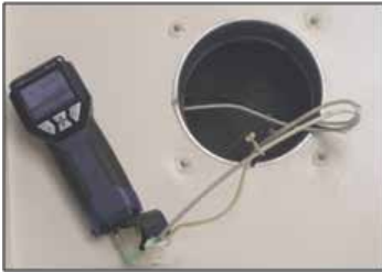
Fig. 18: Example - Connection of the measuring hoses
