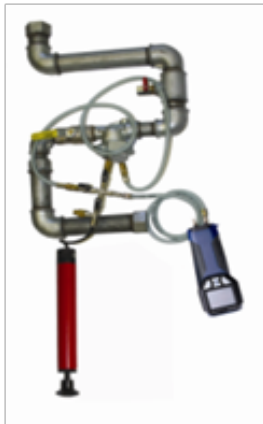
Fig. 54: Volume measurement with the Lindab PC 410 and a syringe (up to 100 ml tube volume).
