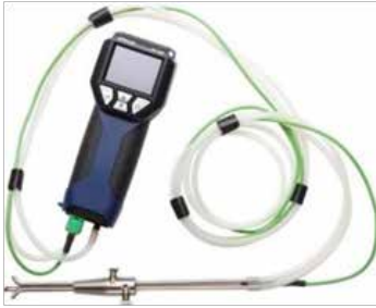
Fig. 34: Connection of the S-tube probe to the PC 410
