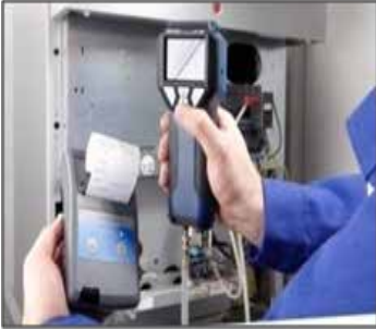
Fig. 60: Transmission of data records from the PC 410 to the thermal fast printer TD 600.
