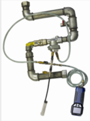
Fig. 53: Volume measurement with the Lindab PC 410 and a syringe (up to 100 ml tube volume).
