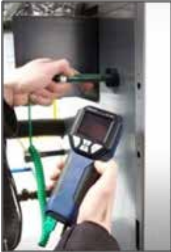
Fig. 57: Application example with Special Wall Temperature Probe
