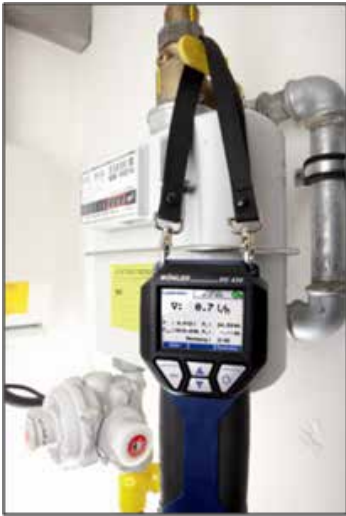
Fig. 16: PC 410 with supporting loop
