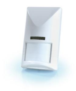
IR24-P is a presence detector designed for automatic ventilation control of HVAC systems. It saves money and gives higher comfort in premises which require forced ventilation for shorter periods of time, such as conference rooms, assembly-halls etx. The unit provides a changeover relay signal output for start/stop of fan or similar equipment. It can be wall or corner mounted with 110°, 15 m detection range.
