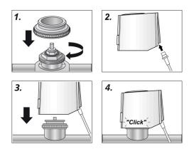
Valve adaption is archived by a valve adapter which is available in different versions to suit the most common valve bottoms and heating circuit distributors (please consider when ordering).
